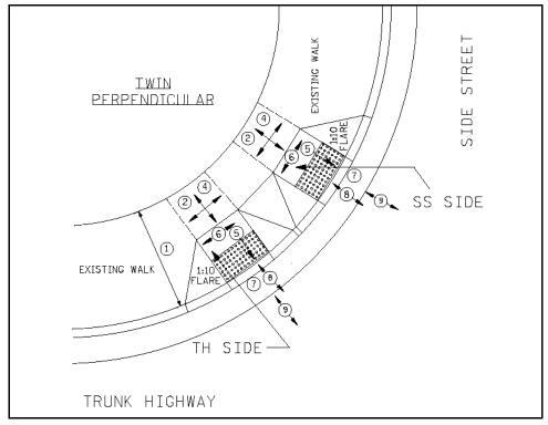
Figure 7 – Twin Perpendicular
