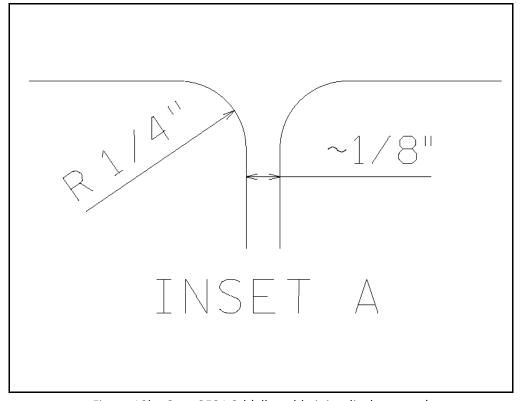
Figure 10b - Spec 2521.3d (allowable joint displacement)
