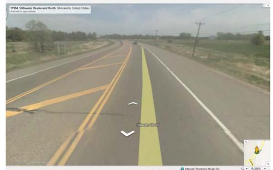
Figure 31 - Twelve-foot buffer with rumble strips
