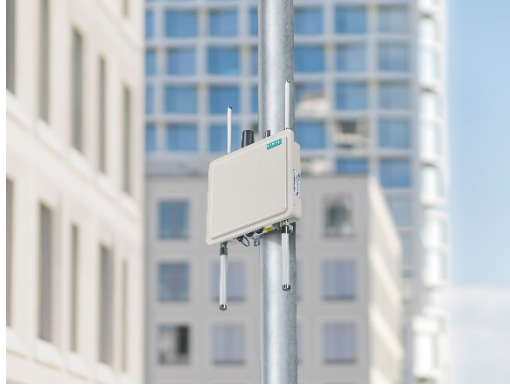
Figure 9. Roadside Unit (RSU) Mounted on Light Pole
