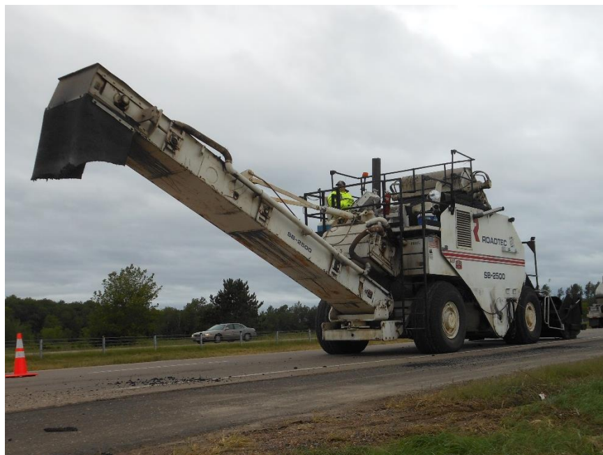
Figure 500.14 – Material Transfer Vehicle from the rear. The area between the front and rear wheels can store and remix several tons of asphalt mixture.
