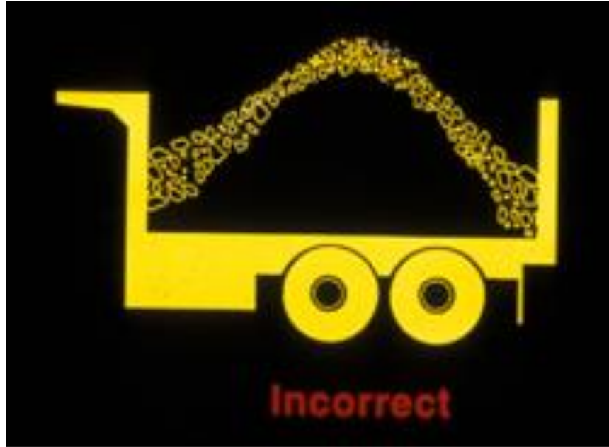
Figure 600.3 – Incorrect loading of asphalt mixture.
