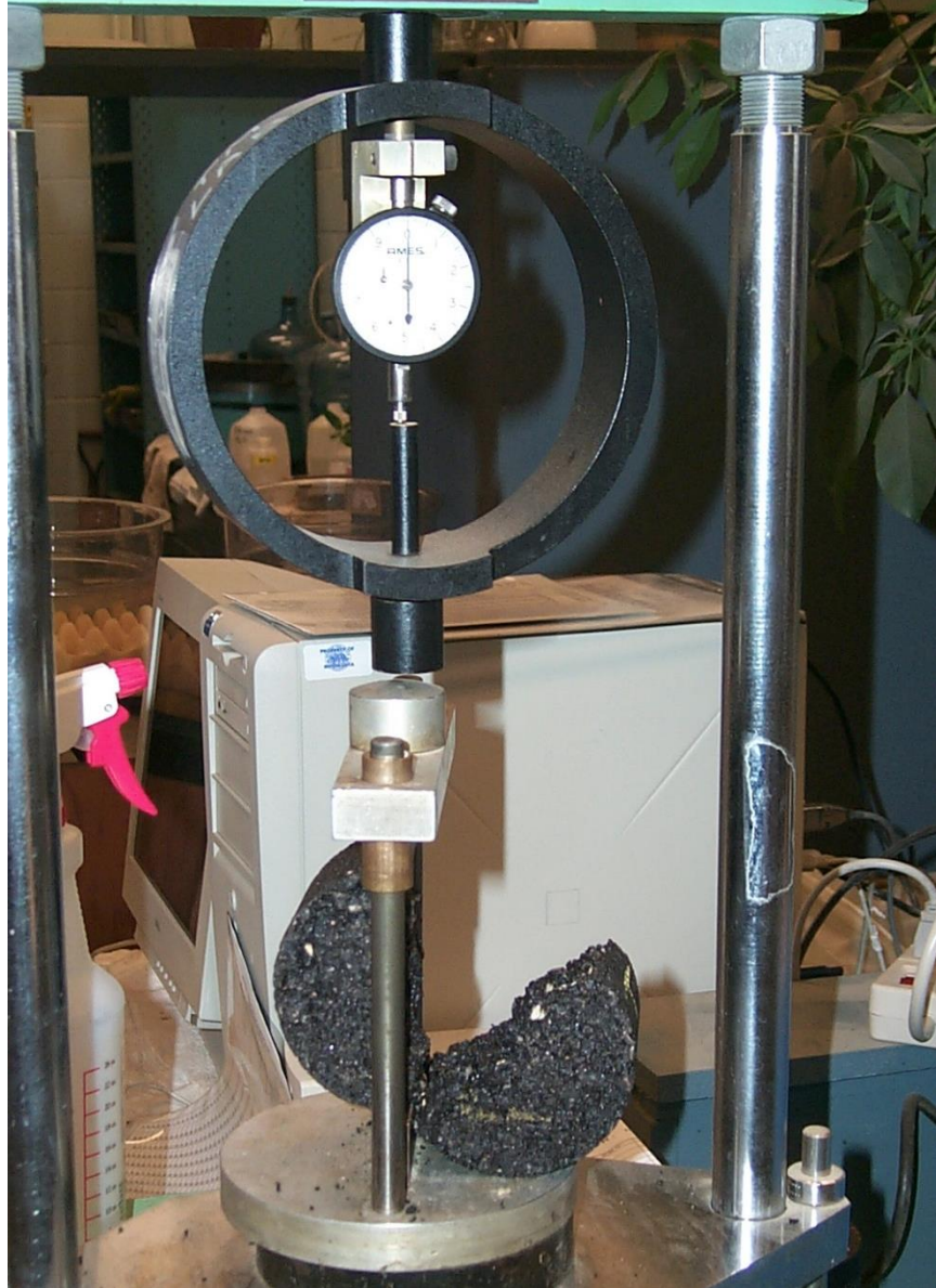
Figure 300.3 – Apparatus used to perform a Lottman test.
