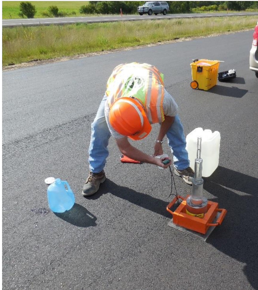
Figure 300.1 – Falling-Head Permeameter used to measure permeability of the mat
