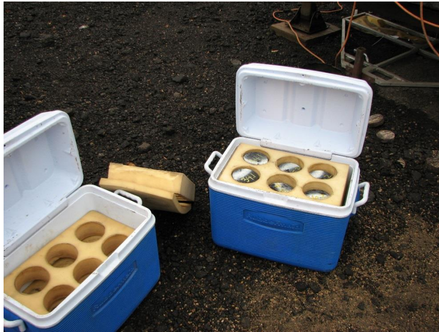
Figure 500.27 – A cooler modified for core transportation. This is an example of good core handling.
