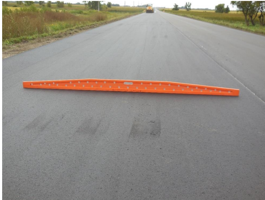
Figure 500.28 – 10-foot Straight Edge
