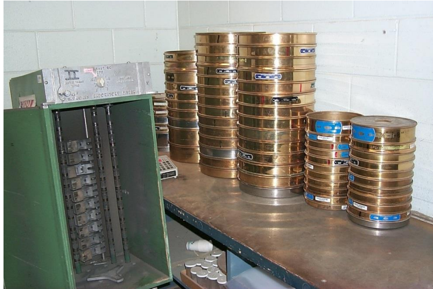
Figure 200.17 – Sieves and sieve shaker used to run an aggregate gradation.
