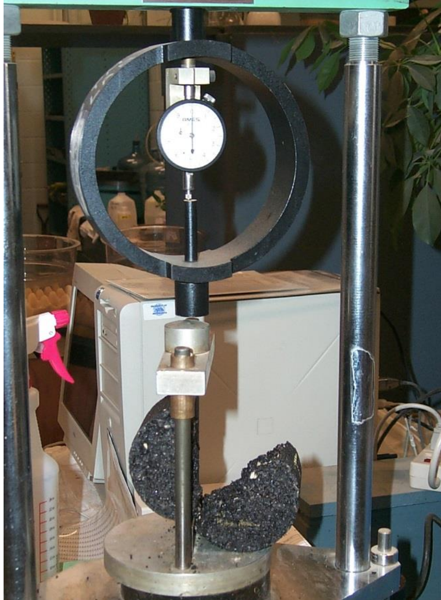
Figure 700.8 – Lottman Load Frame
