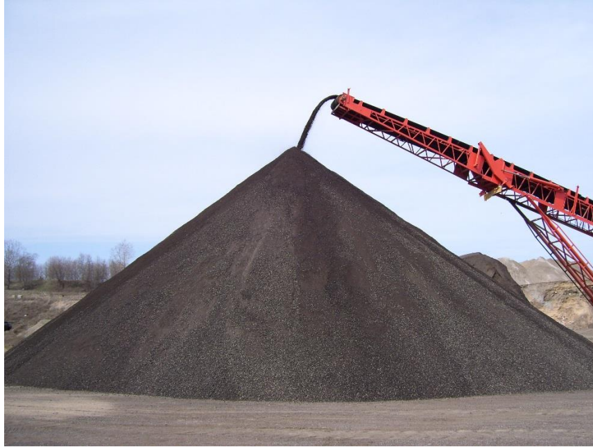
Figure 200.15 – A stockpile of processed RAP
