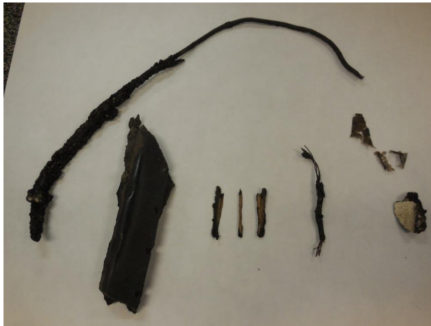
Figure 200.16 – Examples of RAP contaminants including loop detector wires, rubber sealant, and wood
