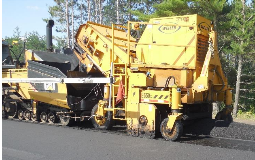
Figure 500.12 – Remixing Pickup Machine. Note the auger bearing just above the point of discharge.
