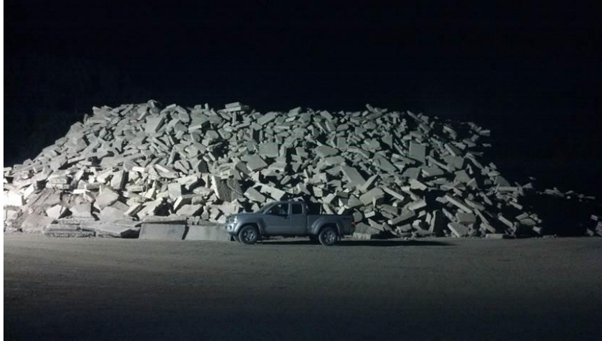
Figure 200.14 – Pile of recycled concrete ready for crushing
