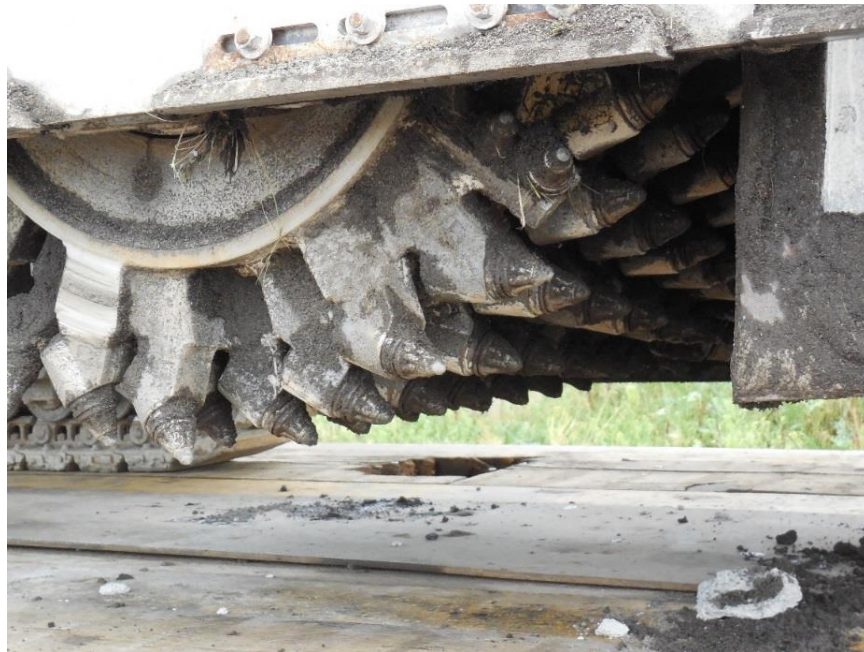
Figure 500.3 – Close up of a micro milling drum. This particular drum is capable of milling 4 feet wide.
