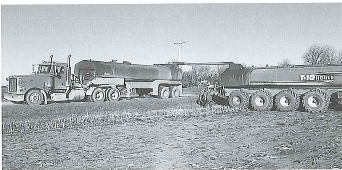
Eisentraut AG sometimes moves materials from farm to field by transferring loads from a tanker on the road to spreaders in the field, avoiding the need to drive a heavier vehicle on town roads.
