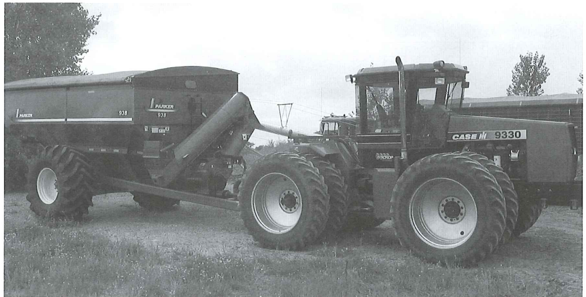
Testers compared farm vehicles like this single-axle grain cart, loaded and empty, to measure pavement deflection and other results. The study found that individual axle weight mattered more than gross vehicle weight in causing pavement failure, suggesting the more axles, the better.
