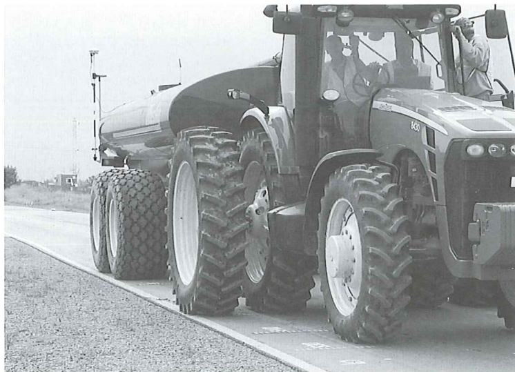
The study measured different load levels over five days of testing on the flexible pavement sections in each of the spring and fall test periods. Experienced drivers drove tankers like this one, empty and with loads at 25, 50, 80 and 100 percent capacity.
