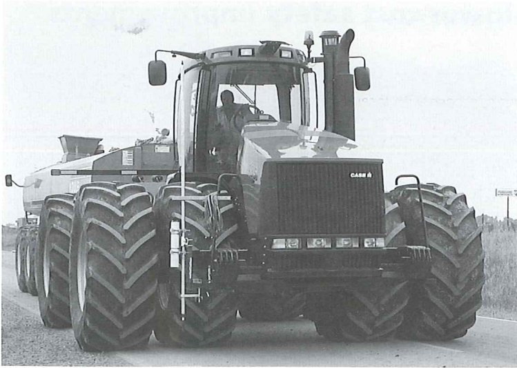
Allowing large tractor tankers transporting agricultural materials, like the 9500-gallon MnROAD test vehicle pictured here, to use temporary one-way routes during hauling operations can protect town roads from serious damage.
